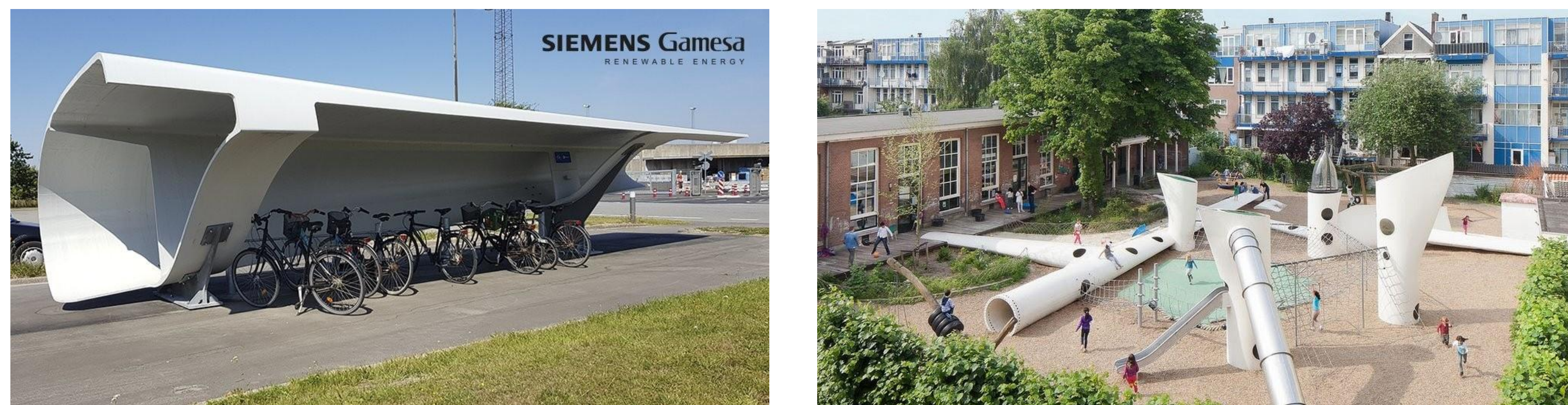
Figure 1. A bike shelter (left) and park (right) in Denmark and Netherlands respectively, both made from decommissioned turbine blades.
